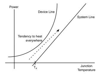
Figure 8. System with NO Operating Point, Overheats as Soon as Powered Up
