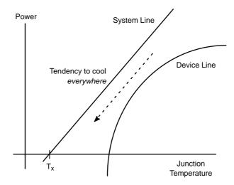
Figure 6. System with No Operating Point, Negative Second Derivative, Cannot be Powered Up
