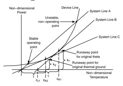
Figure 11. Solution of Device and System Equations in Non-dimensional Coordinate System
