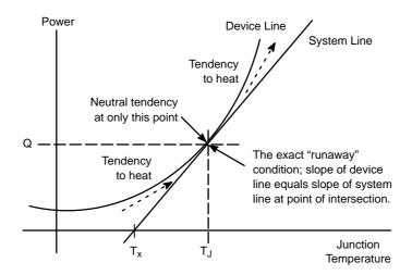
Figure 9. System with Exactly One "Runaway" Operating Point,
